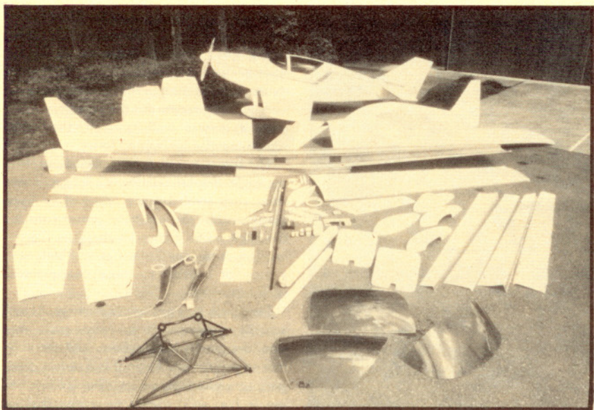
By replacing the plastic with fiberglass composite, the Glasair becomes a grown-up version of a Revell model airplane kit. But when assembly is complete, it will not fit on your mantel.
